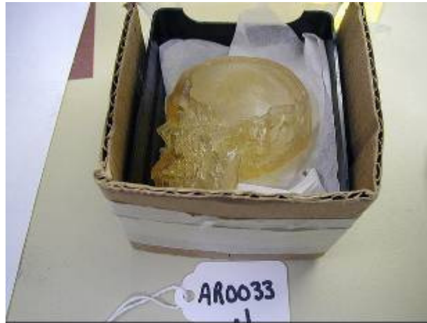
Figure 3 - A “sample” model of a skull from the Walter Reed 3-D Imaging Center. The models are usually full size. They are generated from 2-D medical images (CT scans). This model, one-quarter size, was produced using SLA 7000 stereolithography system from 3D Systems, Valencia, CA, USA. Canada Science and Technology Museum, Artifact no. 2007.0221. Photo by author, 2014.
