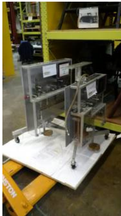
Figure 4 - Part of the Hydrogen Fluoride (HF) absorption cell and gas-handling unit, c. 1981. Now in the warehouse at the Canada Science and Technology Museum. Photo by author, 2104.
