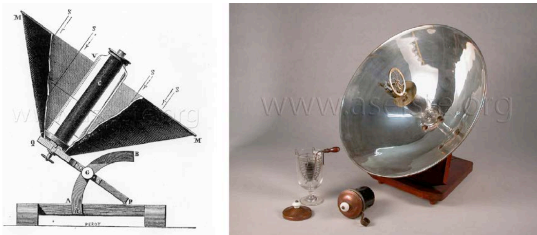
Figure 11 – Mouchot solar driven steam engine. Lycée Guez de Balzac, Angoulême . Instrument maker: Mouchot.
